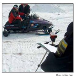
A snowmobile's sound level is being measured by a law enforcement officer using the SAE J2567 stationary sound test.
