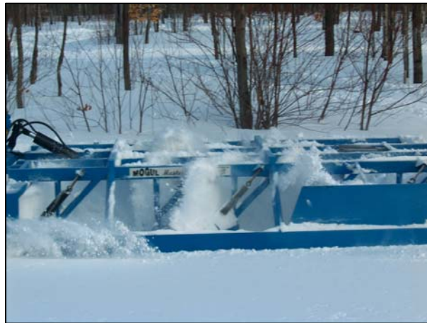
Photo 4.5 Keep processed snow inside the drag!
