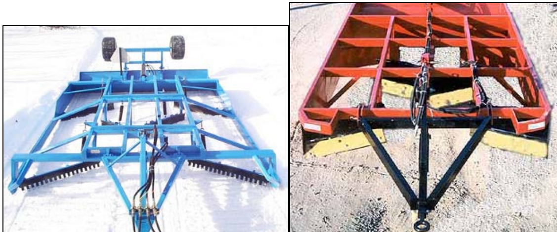
Photo 2.3 Typical multi-blade frames and blade configurations
