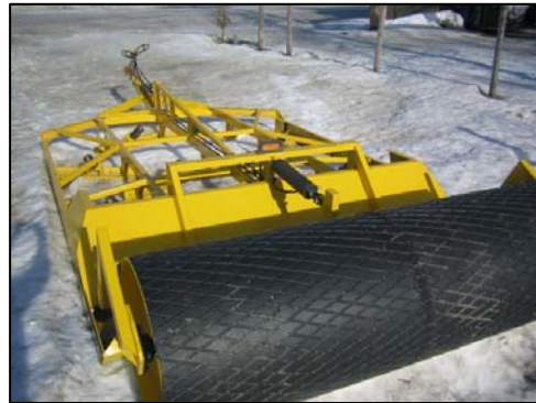
Photo 2.16 Typical rear drum roller assembly
