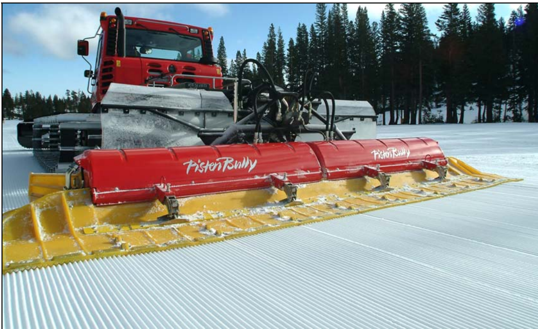
Photo 2.22 Flex tiller set in a rigid (straight) position with lockout device shown below.
